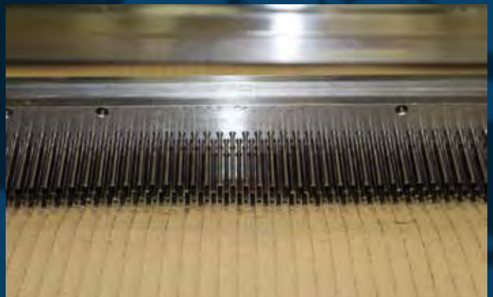
Image of a perforating tool with four rows of punches. Closeup of partial tool shown for detail.
