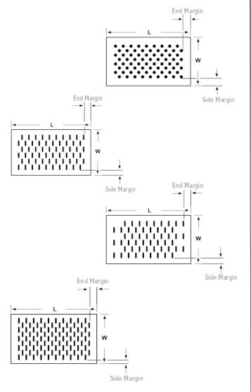
All perforated sheets require blank areas. According to the application, user should give the dimension and location of blank area(s).
