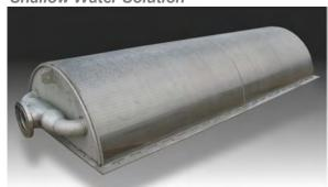
For shallow water conditions, Hendrick offers a patented halfbarrel intake screen. With the same flow characteristics of our T-Intake screens, the bottom discharge outlet allows complete functionality in low water. Ideal for shallow creeks or rivers where a full T-Intake screen won't work.
